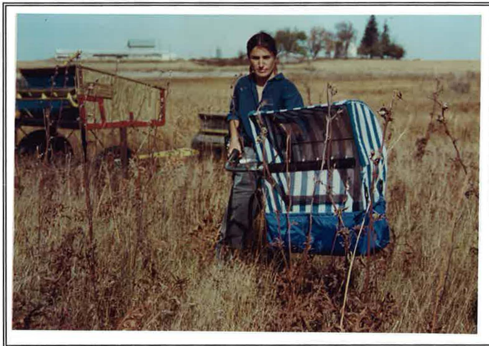
The medium technology, power seed stripper - a new use of your basic weed whip.
