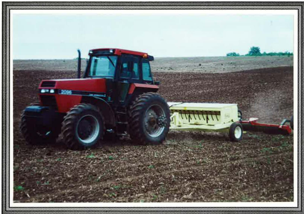
A variety of planting techniques were used in 1995, including this Truax broadcast drill.
