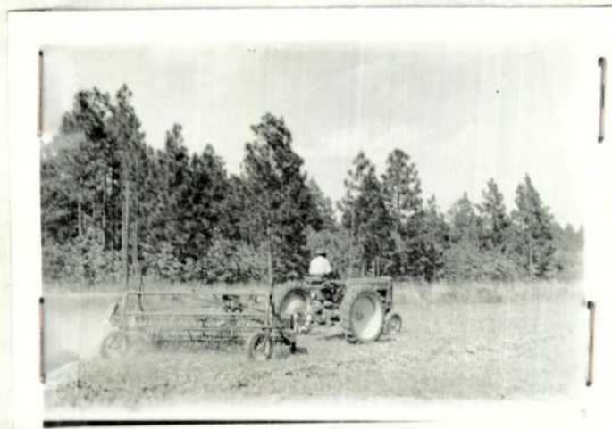
Side delivery rake in operation removing weeds from serocia field after mowing.
