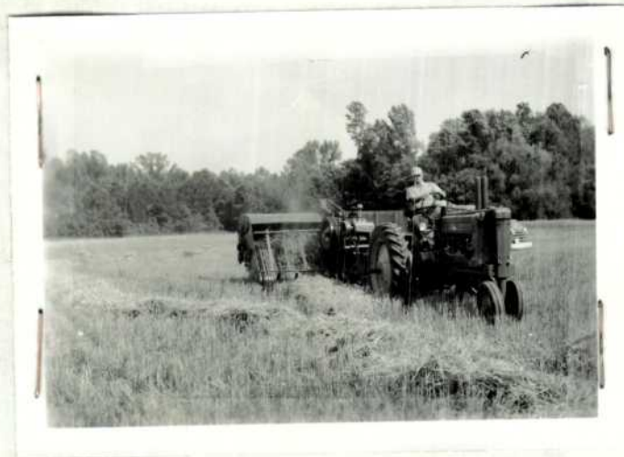
Pickup hay baler in operation removing wheat straw from land seeded to lespedeza.
